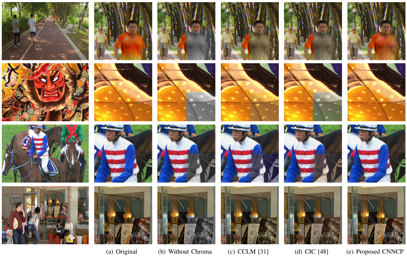
Fig. 8. Chroma prediction performance comparison with images from VVC sequences, and the blocks located at the bottom-right are predicted. From top to bottom, the sequence indicates ParkRunning3, NebutaFestival, RaceHorsesC, and BQMall, respectively. The PSNR values are illustrated in Table IV.
